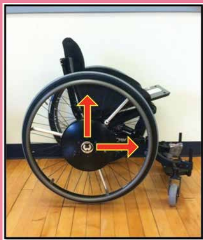
FIGURE 2 REAR AXLE POSITION (RAP) - Moving RAP up and forward relative to shoulder can improve propulsion biomechanics
