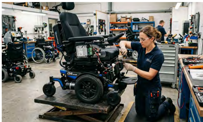
Technician testing electronics and making repairs in shop.
