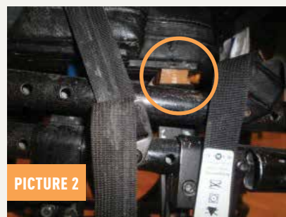
Picture 2: Polymer between the seat rail and seat mounting hardware.
