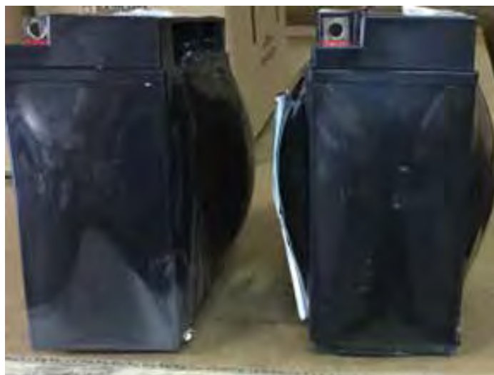
Figure 3: Bloating Battery Example
