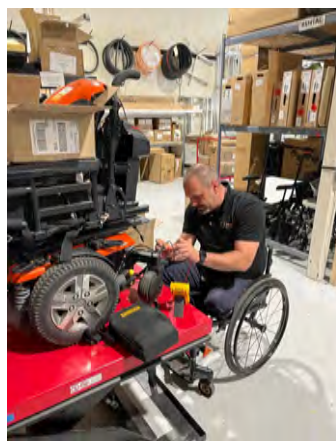
Matthew Pritchett, RRTS®, troubleshoots electrical issues with a Quantum power chair.
