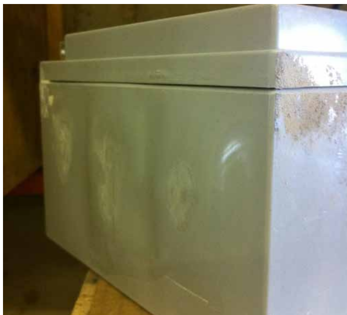
Figure 4: Rippled Battery Example
