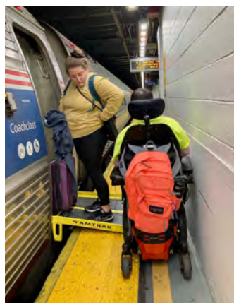
Figure 3: Poor bridge plate accessibility to enter an Amtrak train car.
