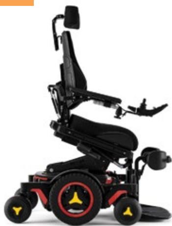
FIGURE 1: Permobil M3 with 20 degrees of active reach combining power seat elevation, anterior tilt, recline and leg rests.
