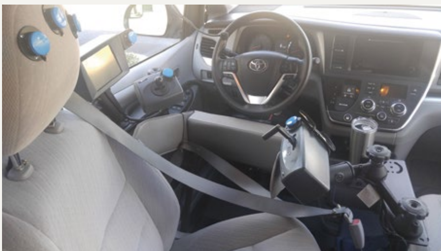
This setup shows the equipment that Romano uses to drive independently.
