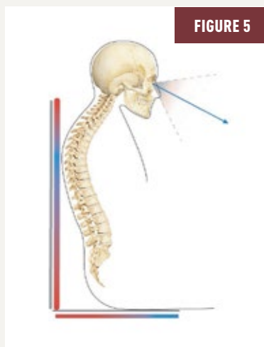
A 90-degree seat-to-back angle can result in posterior pelvic tilt, kyphosis and a downward gaze
