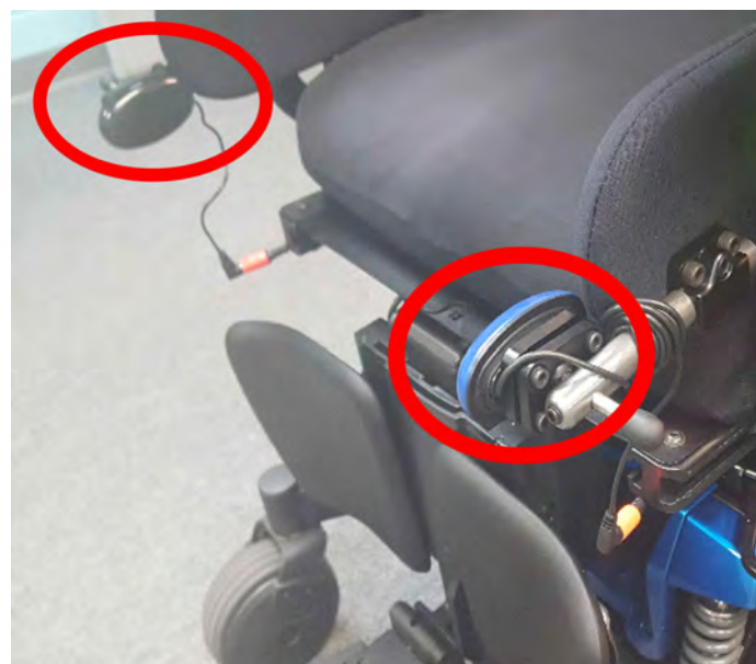
Linked driving setup with mechanical switches mounted at lateral knees for access.
