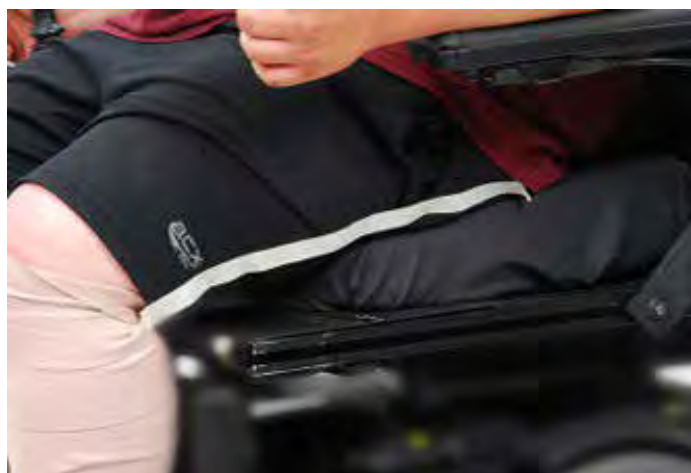
Rigid edge of the power wheelchair base exposed due to insufficient cushion depth, resulting in circulatory problems and ischemic skin changes in the lower limbs.
