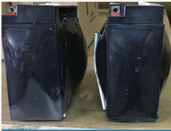
FIGURE 7 Bloated battery examples
