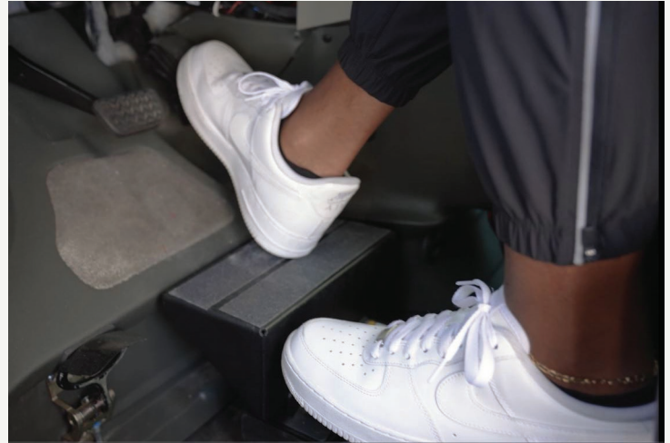
PHOTO 4 Removable platform to provide foot stability while accessing gas and brake
