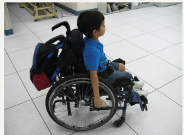
FIGURE 1 Josh in his first wheelchair when I met him. Note how far back the center of gravity is.
