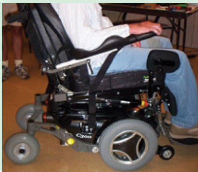
FIGURE 1 Front-Wheel Configuration: The drive wheels are in the front.
