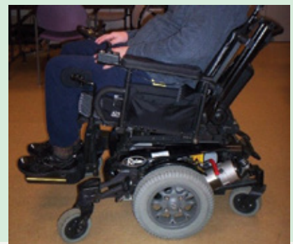
FIGURE 3 Mid-Wheel Configuration: The drive wheels are in the middle.
