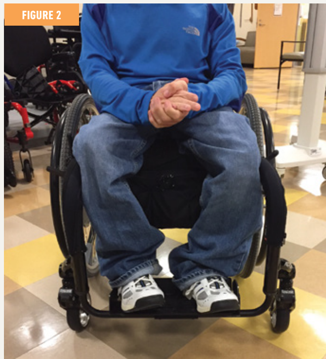
FIGURE 2: This shows the front caster wheel sticking out further than the rear wheel. This was done to allow the chair to track properly when moving forward. The front caster angles are equal on both sides.
