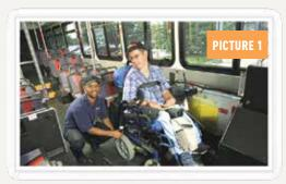
compliant with WC-19 are safe for use as a motor vehicle seat in personal smaller vehicles, as well as in larger public buses. These wheelchairs have been sled impact tested (crash tested) and are equipped with securement points that interface with four-point strap type tie-down systems and are rated for their ability to accommodate proper lap and shoulder belt fit. A list of RESNA WC-19 certified wheelchairs can be found at: <a href="http://bit.ly/2dbw2Iz">http://bit.ly/2dbw2Iz</a>
